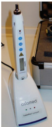
Fig. 1. Laserpen (70 mW, 785 nm, cw laser), Reimers & Janssen, Berlin, Germany Fig. 2. 8 Hz, oscillating between 50 mW and 100 mW; 4 Hz oscillating between 0 and 50 mW
